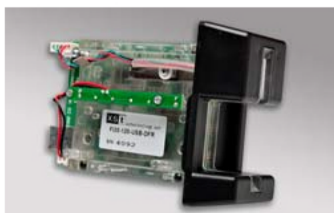
FI30-120-USB Full stripe insert card reader Reads ANSI/ISO tracks 1 and 2 Clear module with illumination USB 1.0/2.0Mb/s interface
