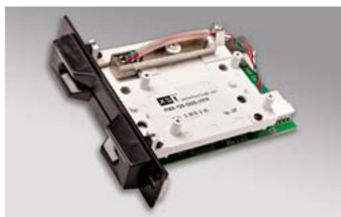
PI65-120-GDS Partial stripe insert card reader Reads 65% of track 1 and 2 Bit/Strobe interface USB/HID interface
